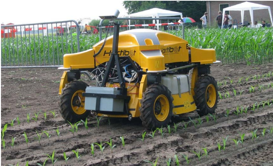
Figure 4 "Hortibot" is an autonomous plant nursing robot that can control weed efficiently (Source: www.hortibot.dk )
